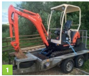
1 Mini excavator used for internal trial holes
